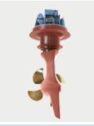
The streamlined leg and skeg recover swirl energy from the slipstream, raising the overall propulsive efficiency. The leg has a wide chord to optimise rudder effect and improve the vessel's course stability.
