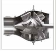
The impeller's task is to pressurise the water. The reaction force that is created when the water leaves the pump is utilised to propel the ship.
